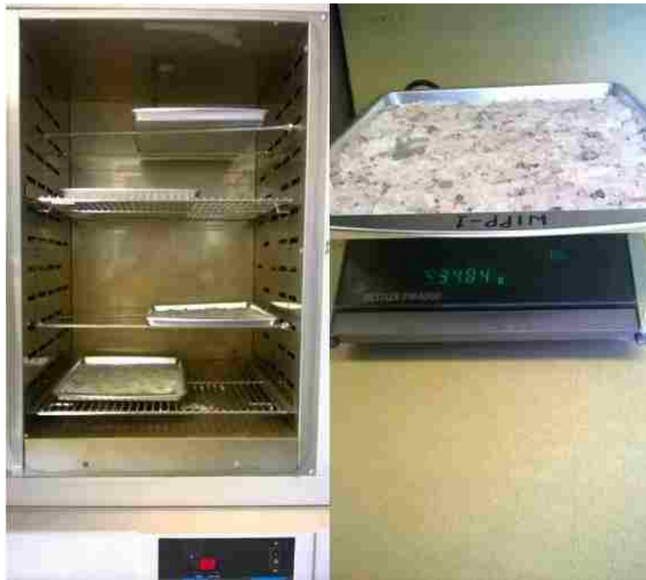
Figure A1 Granular salt placed inside the oven (left) and a digital weighing machine measuring the mass of salt.
